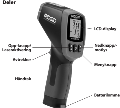
Figur 2 – mikro IR-100, deler
