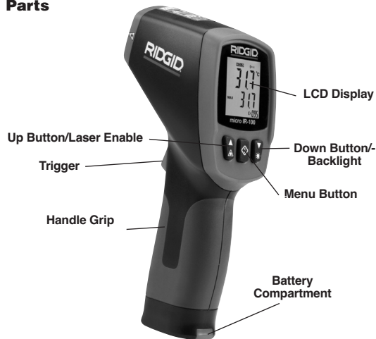
Figure 2 – micro IR-100 Parts
