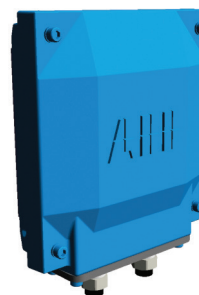
Auxiliary cast iron terminal box Frame size for motor sizes 160 - 250 (variant code 418): 119 x 170 mm, max. 18 strips. No earthing.
