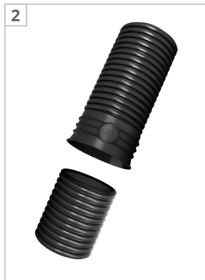
2. The pipes are connected by means of sockets on pipes or pipe fittings. An elastomeric gasket is required to seal the connections.
