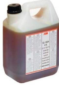
IG 1601, IG 1604 Insulating oil, for joints and terminations for paper-insulated cables 12-52 kV. Need not be heated at temperatures exceeding +10°C.
