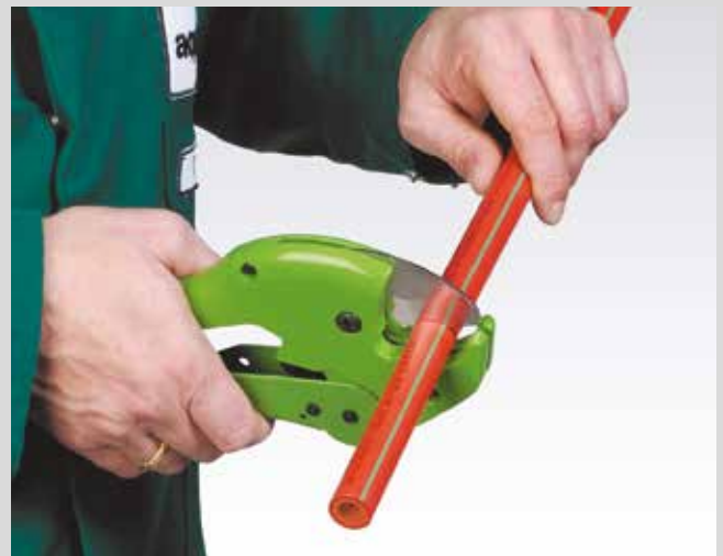
Cutting of the pipe
