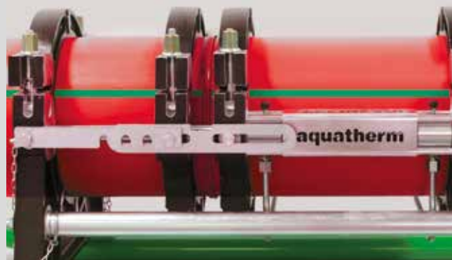
Join the pipes, cool down under pressure
