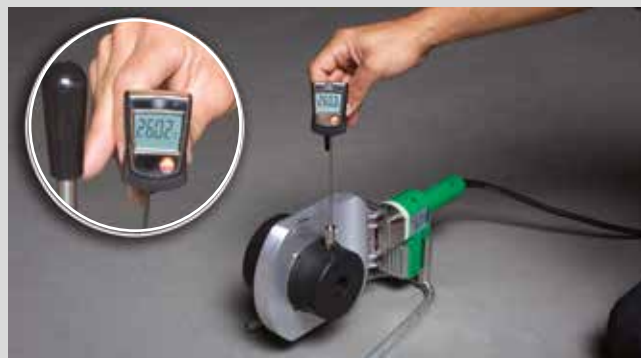
Temperature control aquatherm welding device (1400 W)
